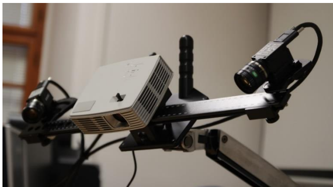
3D skener (HP 3D Structured Light Scanner)
